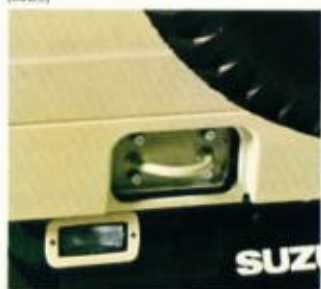
Towing bar & foot step (LJ20, LJ20V)
