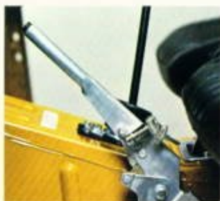
Parking brake with anti-theft locking device (LJ20)
