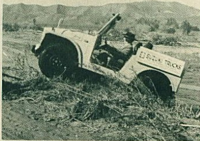
Suspension provided jouncy but not teeth jarring rides, even over rough terrain like this. The response was so quick that unexpected bumps could be met with proper speed and angle of approach.
